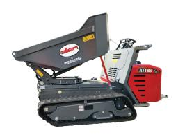
The AT19S is the largest all-new Allen track buggy. Designed for professional contractors, this reliable equipment boasts precise maneuvering capabilities and topnotch performance. The sturdy steel bucket with a 90-degree dump angle and 180-degree pivoting dump ensures accurate material placement, allowing you to achieve superior results every time.
